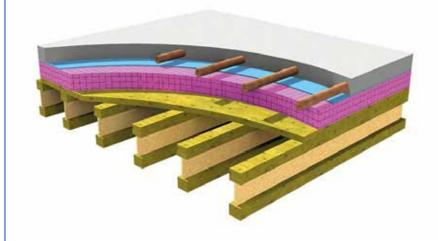
40mm (allow minimum 25mm cover to pipes) of **GYPSOL** TimBRE Screed with embedded underfloor heating Optional thermal or acoustic insulation 500g polythene slip membrane 22mm OSB deck
