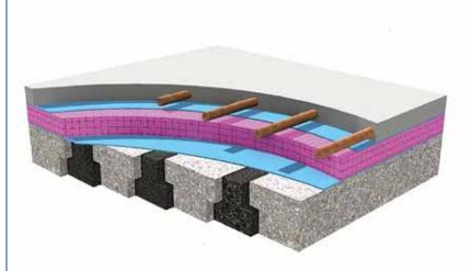
40mm (allow minimum 25mm cover to pipes) of **GYPSOL** TimBRE screed with embedded underfloor heating Minimum 500g slip membrane Minimum EPS100 polystyrene insulation Minimum 1200g polythene damp proof membrane Beam and block or ground borne concrete substrate as appropriate
